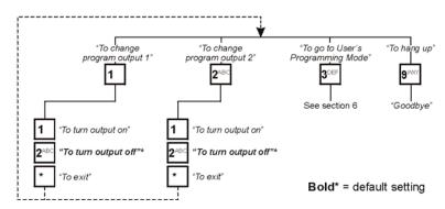
The User's Opening Menu allows you to activate or deactivate the programmable outputs. The programmable outputs (PGM1 & PGM2) can be used for remote switching of other devices. For example, a PGM can be used to turn on air conditioning or heat, extinguish lights, activate a sprinkler system, or open a garage door. Speak to your installer for more information.
