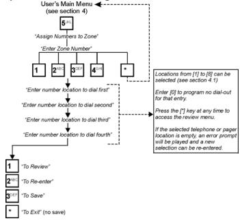
The ParaVox can assign up to four telephone numbers or 4 pager numbers to each of the four zone inputs. This means each zone has a prioritized sequence of dialouts customized to suit the input. Since voice and pager messages are linked to specific zones, telephone numbers assigned to a zone will play the same voice
