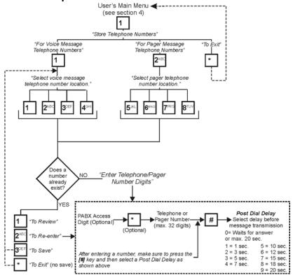
The ParaVox unit can store up to four telephone numbers in locations [1] to [4] and up to four pager numbers in location numbers [5] to [8]. When a telephone number location is assigned to a zone (see *Telephone Number Assignment* on page 12), the ParaVox will dial the number programmed here whenever the zone is triggered. The telephone numbers are programmed into the desired locations as described above.
