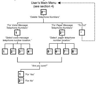
Previously stored voice message telephone numbers and pager telephone numbers can be deleted by entering option [1] or [2] from the Delete Telephone Numbers menu. Select the desired voice message telephone or pager number location. Deletion is confirmed by entering [1] for yes or [2] for no.
