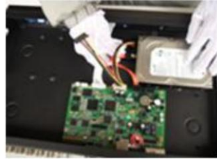
②HDD data line and power line connection
